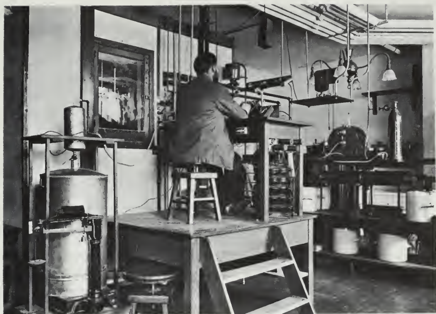
The Atwater-Rosa respiration calorimeter, the first successful instrument designed to measure the energy requirements of people, was moved from the University of Connecticut to the Department of Agriculture in 1908.
